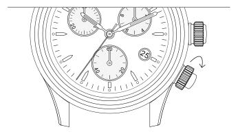
**RESET BUTTON:** Unscrew the pusher counterclockwise and press when resetting the chronograph. Make sure that the push button is tightened after using the functions of the chronograph. Do not use the pushers while submerged under water.
