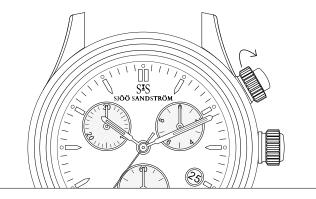
START/STOP BUTTON: Unscrew the pusher counterclockwise and press when starting/stopping the chronograph. Make sure that the push button is tightened after using the functions of the chronograph. Do not use the pushers while submerged under water.
